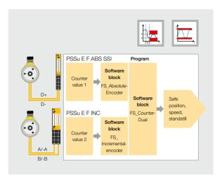
Safe speed, safe position - with two encoders.
