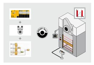
Safe electronic rotary cam arrangement – approved safety solution compliant with EN 692.
